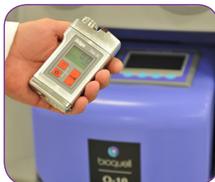
Image 2. Hand held HPV environmental monitoring device provided as standard
